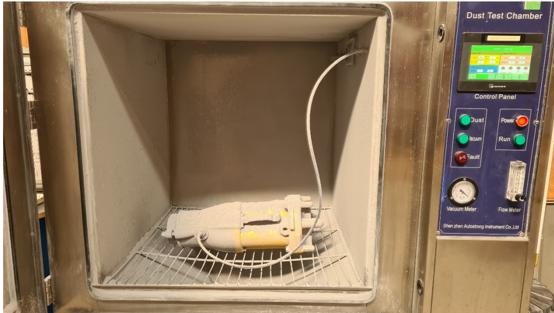
Picture 3 Coupler in dust test
