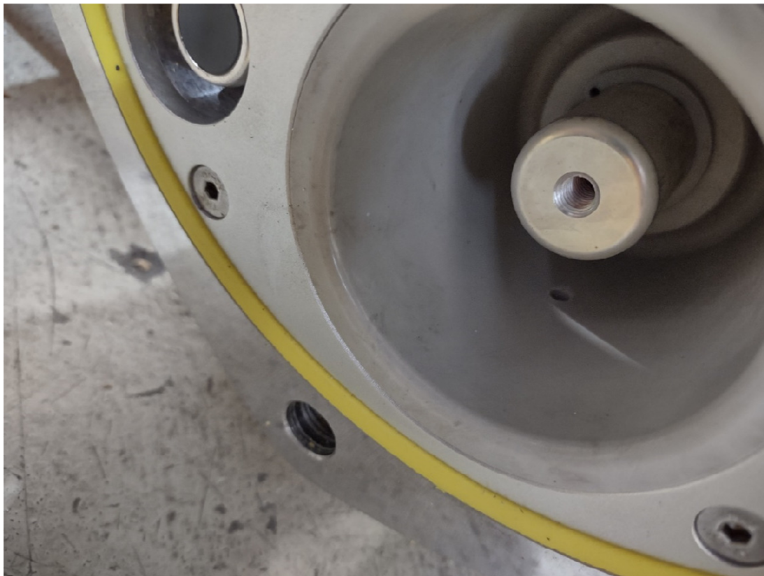
Picture 6 Contacts after short circuit test
