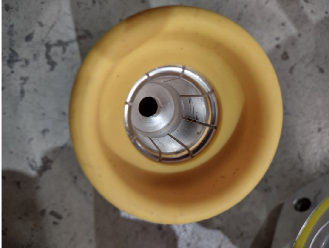
Picture 5 Contacts after short circuit test
