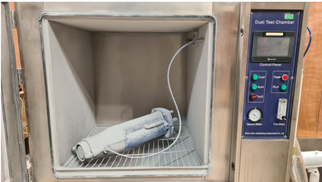
Picture 2 Coupler in dust test
