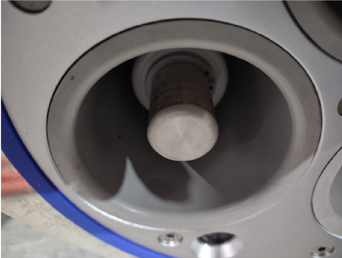
Picture 4 Contacts after short circuit test
