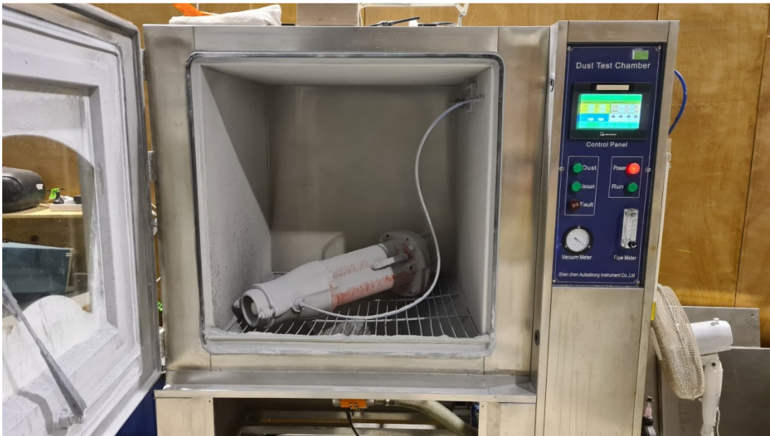
Picture 2 Coupler in dust test
