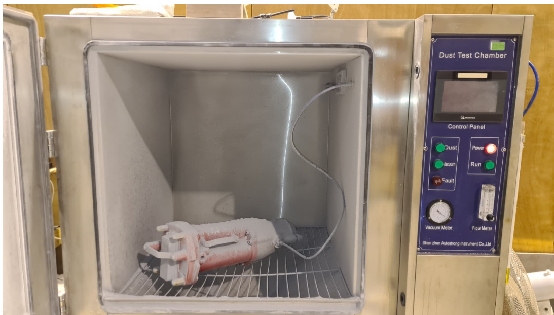
Picture 2 Coupler in dust test
