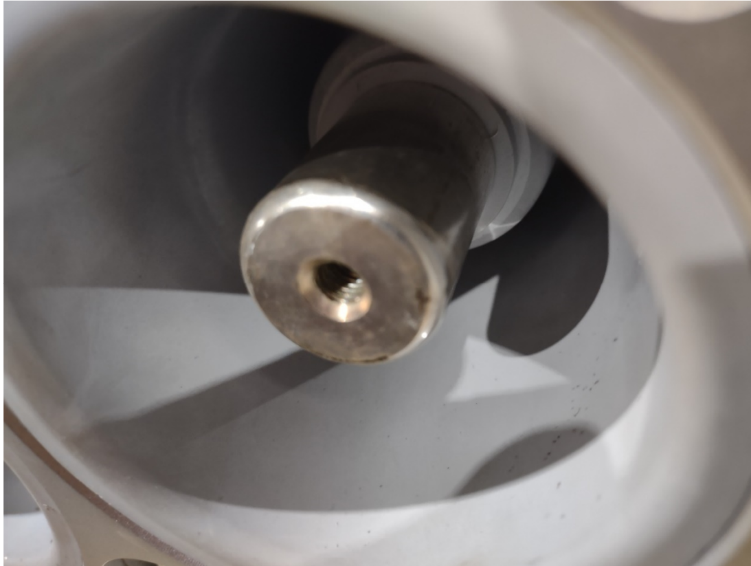
Picture 5 Contacts after short circuit test
